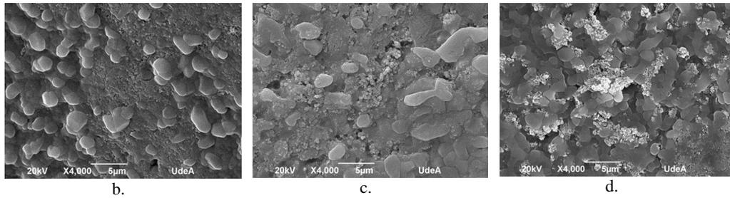
**Fig. 2.** SEM images of a. Pure Hitec, b,c, and, d the MSBNFs after MDSC with 0.5, 1.0, and 1.5 wt.% of alumina nanoparticles, respectively.
