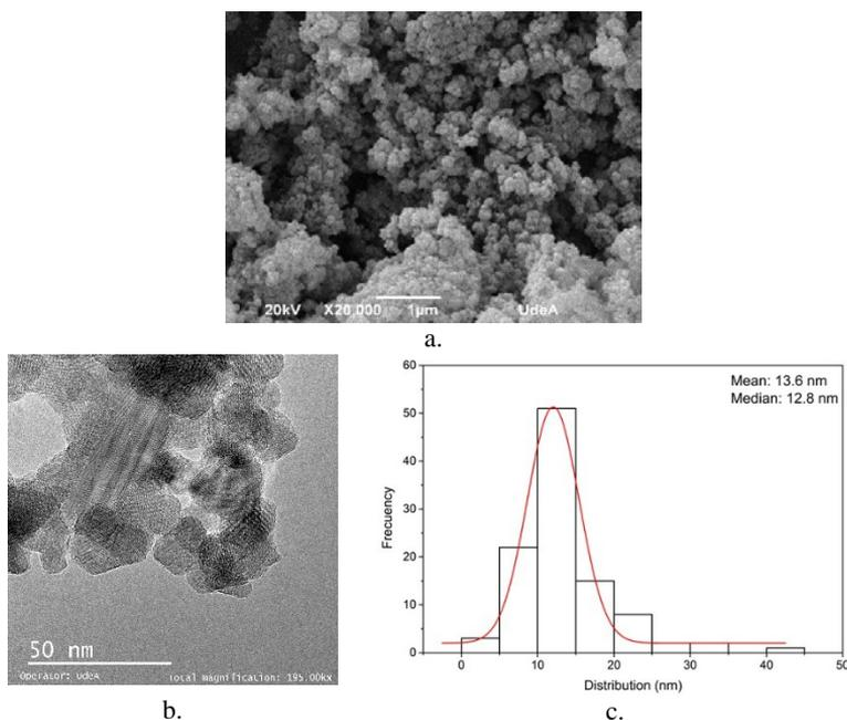
**Fig. 1.** The pristine alumina nanoparticles used to elaborate the MSBNFs. a. SEM image, b. TEM image and c. the size distribution obtained from TEM images
