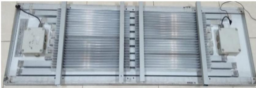
Fig. 5. Solar panel with passive cooling device
