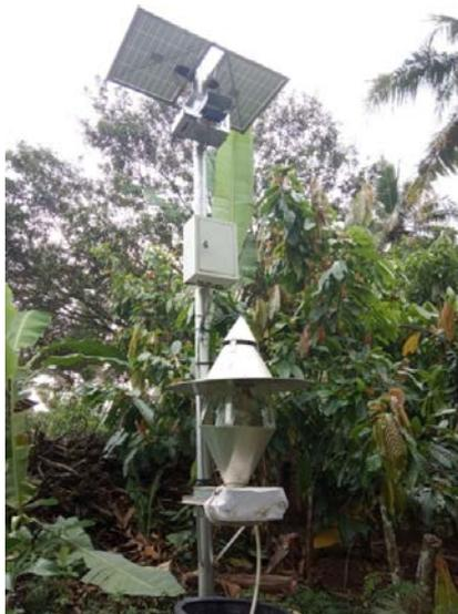
**Fig. 4.** The automatic insect trap in cacao plantation
