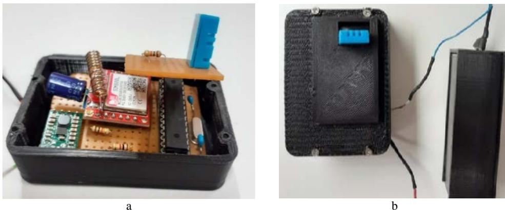
Fig. 7. Prototype of the traceability system: a) – Prototyping board; b) – System box
