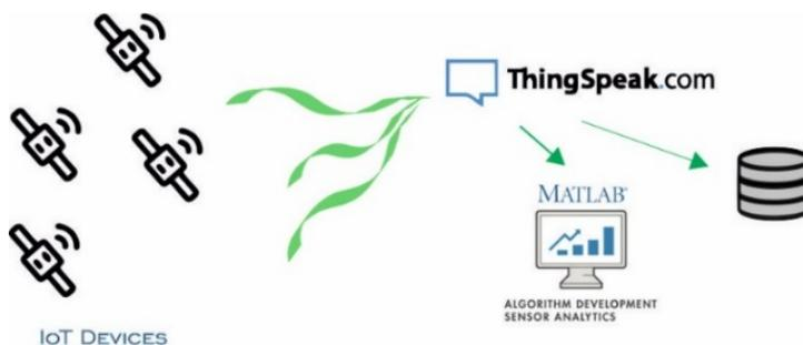
Fig. 5. Illustration of the communication flow between the data sent by the IoT devices and the ThingSpeak server.
