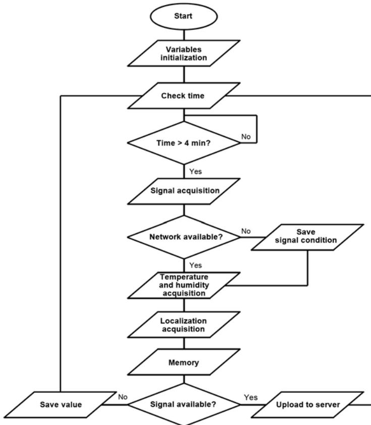
Fig. 4. Flowchart of the operation of the monitoring device.
