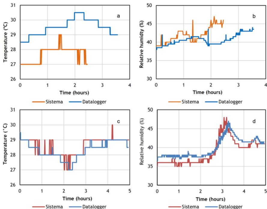
**Fig. 8.** Comparison of measurement values between the Datalogger and the developed monitoring system: a) Temperature monitoring values (without offset); b) Relative humidity monitoring values (without offset); c) Temperature monitoring values (with offset); d) Relative humidity monitoring values (with offset)
