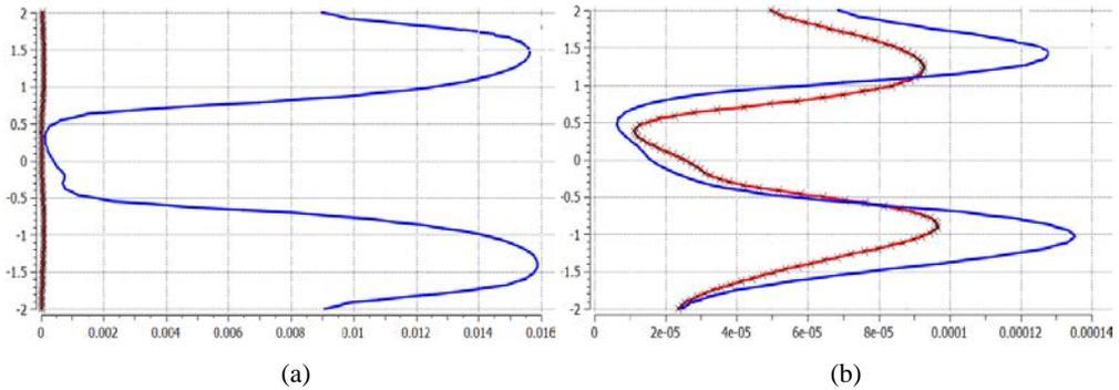
**Fig 4.** The NO<sub>x</sub> content in fuel combustion products: (a) red line – combined combustion of natural gas and biogas; blue line – burning of natural gas; (b) red line – combined combustion of natural gas and biogas; blue line – burning of biogas. Abscissa - Mass Fraction of Pollutant NO<sub>x</sub>, ordinate – vertical flame section
