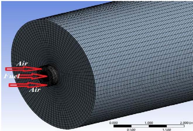
Fig 1. Meshing cylindrical combustion chamber
