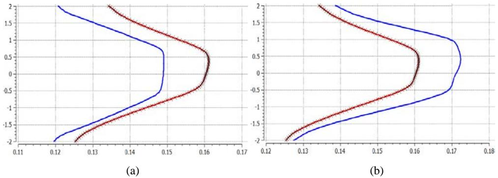
**Fig 5.** The CO<sub>2</sub> content in fuel combustion products: (a) red line – combined combustion of natural gas and biogas; blue line – burning of natural gas; (b) red line – combined combustion of natural gas and biogas; blue line – burning of biogas. Abscissa - Mass Fraction of Pollutant CO<sub>2</sub>, ordinate – vertical flame section
