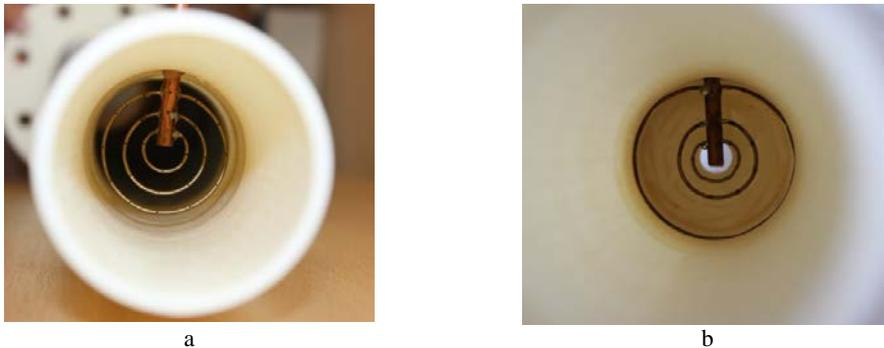
**Fig. 6.** Experimental model of fuel distribution element: a) axial fuel injection; b) combined axial and radial fuel injection
