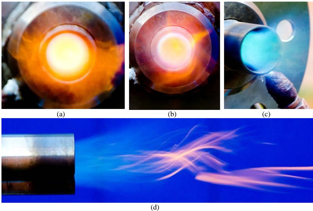
Fig. 4. The photographs of the combustion for the “liquid-to-gas” transition: (a) kerosene combustion; (b) kerosene combustion mainly ( $g_{ker} = 0.75$ ); (c) propane combustion; (d) propane combustion mainly ( $g_{ker} = 0.16$ )
