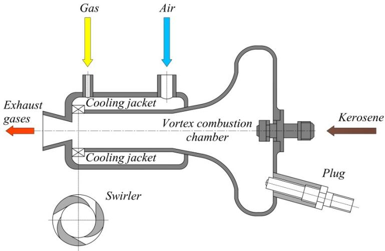
**Fig. 1.** Bidirectional vortex combustor
