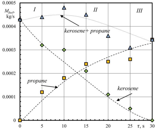
Fig. 3. The dependence of fuel mass flow rate on time for the “liquid-to-gas” transition
