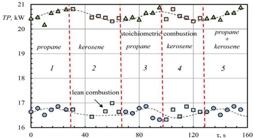
**Fig. 8.** Consecutive transitions between the multifuel operation modes of the combustor
