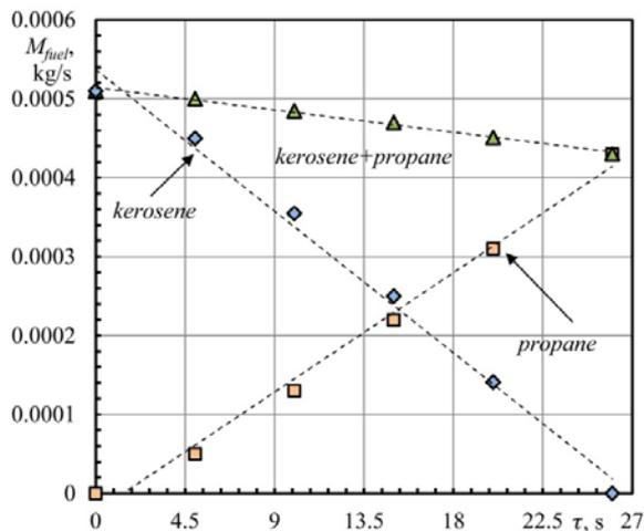
**Fig. 5.** The dependence of fuel mass flow rate on time for the “liquid-to-gas” transition after calibration of needle valves
