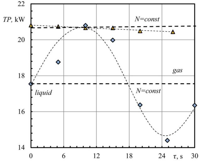
Fig. 6. The total thermal power of the bidirectional vortex combustor for the “liquid-to-gas” transition
