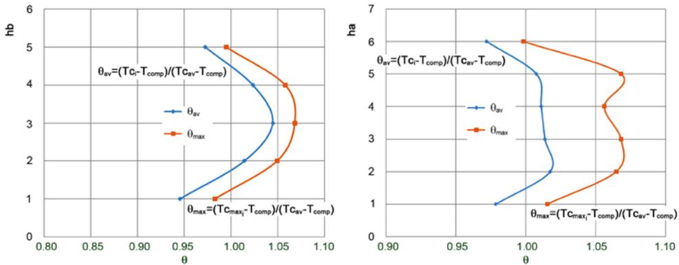
Fig. 6. The unevenness of the temperature field at the cut: left – along the height and right – around the circumference
