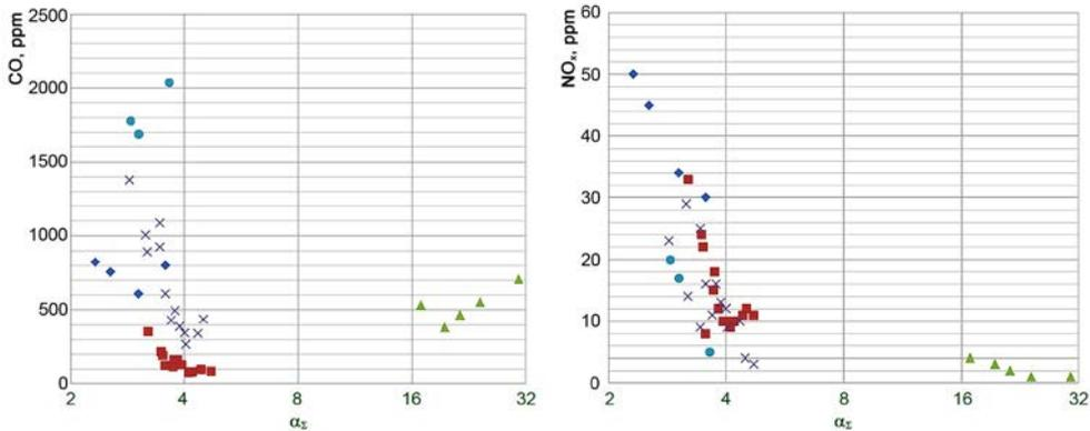
**Fig.4.** Emissions of CO (left) and NOx (right) for different equivalence ratio in the combustor
