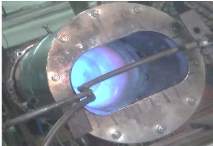
**Fig.2.** Photo of the combustor for sampling combustion products in the optimal mode.
