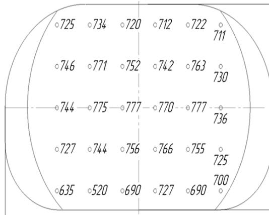
Fig. 5. Outlet temperature distribution in °C,  $G_a=220$  g/s,  $T_{comp}=423$  K,  $\alpha_\Sigma = 3.5$ .
