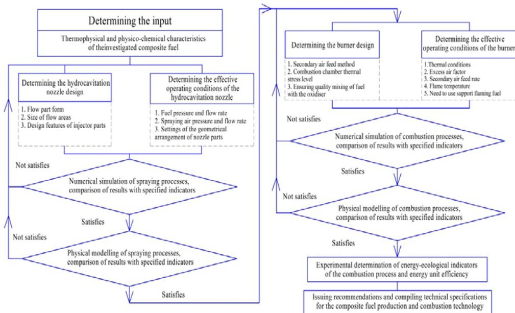
**Fig.2.** Algorithm for choosing (developing) HCA devices and their operating conditions for effective combustion of composite fuel
