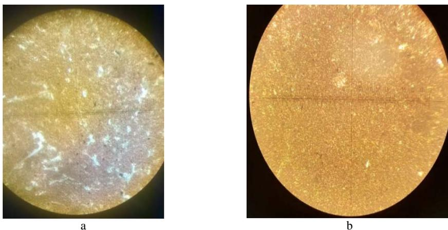
**Fig.4.** Micro photographs of ACLF samples containing a 20 % concentrate of HF flowback water: a) – ACLF obtained on basic equipment; b) – ACLF obtained following the upgrading of the hydrocavitation device and choosing optimal operating conditions
