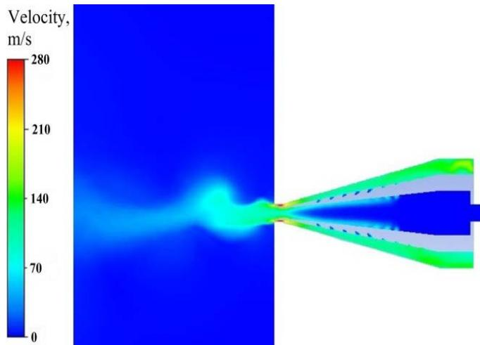
**Fig. 5.** Distribution of two-phase flow rates during composite fuel spraying
