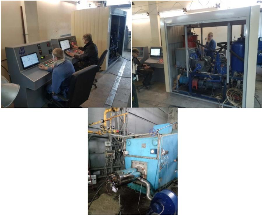
**Fig.7.** Experimental energy-technological complex for research in the processes of producing and combusting composite fuel
