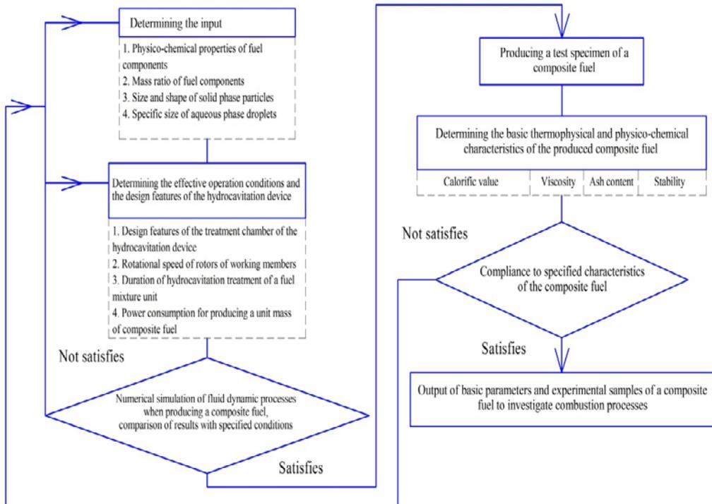
Fig.1. Algorithm for determining HCA effectiveness when producing a composite fuel
