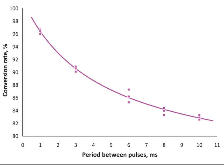
**Fig. 3** Dependence of the conversion rate of sulphur dioxide on the applied voltage pulse period: the initial concentration of sulphur dioxide  $0.61 \text{ g/m}^3$ , voltage 45 kV
