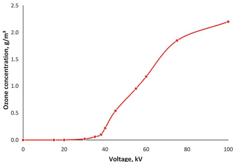
**Fig. 2** Dependence of ozone concentration on the voltage of streamer discharge: pulse period - 1 ms, pulse duration - 200 ns
