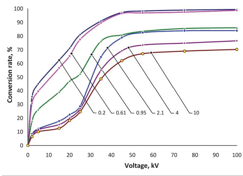
**Fig.1** Dependence of the conversion rate of sulphur dioxide on the voltage of the streamer discharge at different initial concentrations of sulphur dioxide: pulse period 1 ms; pulse duration 200 ns.
