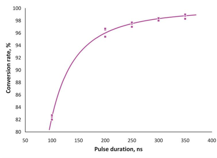
**Fig. 4** Dependence of the conversion rate of sulphur dioxide on the pulse duration: voltage 45 kV; pulse period 1ms; initial concentration of sulphur dioxide  $0.61 \text{ g/m}^3$
