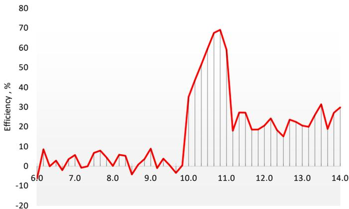
Fig. 8. The efficiency of adaptive regulation based on exhaust gas emission criteria
