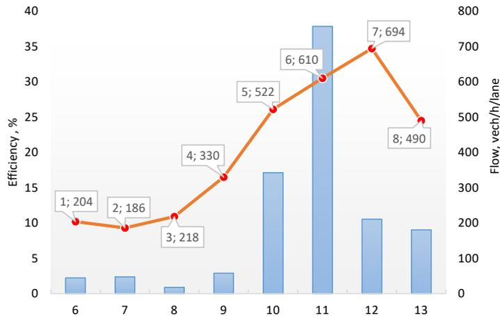
Fig. 9. The efficiency of adaptive control and the relative loading of traffic lanes
