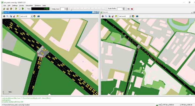
**Fig. 2.** Geo-SUMO intersection model with a geographical sub-base from OSM
