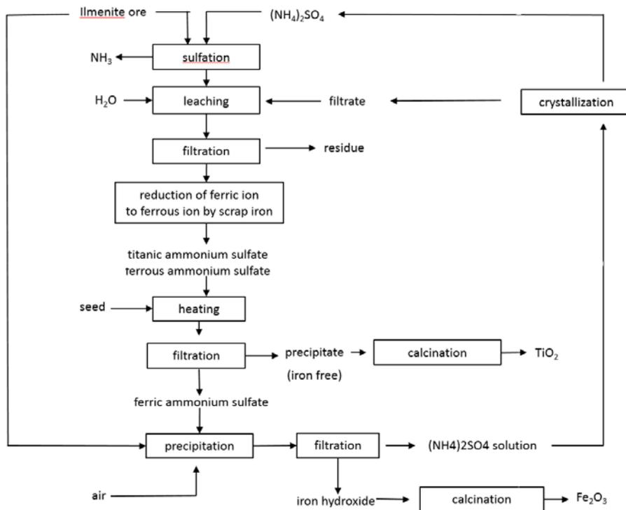
Fig. 2. Technological scheme of producing  $TiO_2$  from ilmenite
