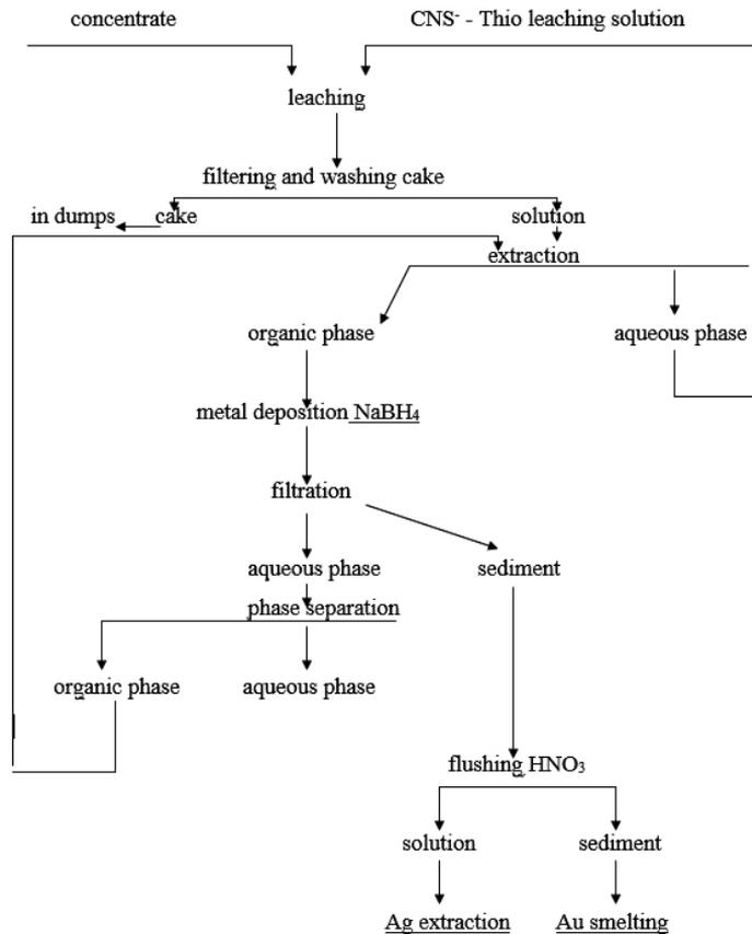
Fig. 3. Hydrometallurgical scheme for the recovery of gold
