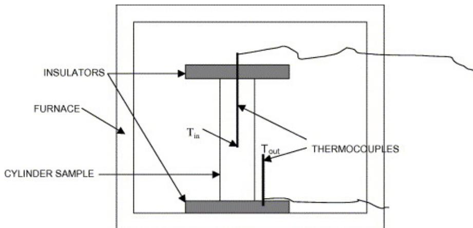
**Fig. 3.** Experimental set-up for fire resistance test
