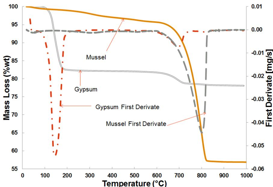
Fig. 4. Mass loss and TG first derivative of raw materials
