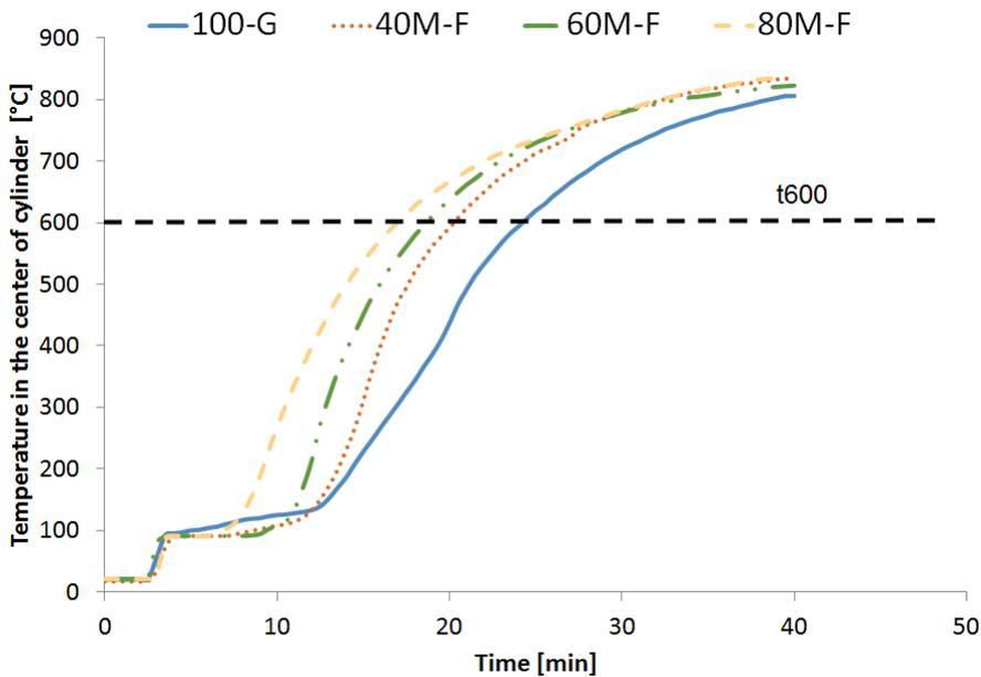
Fig. 5. Fire-insulating capacity of 100-G, 40M-F, 60M-F, 80M-F materials
