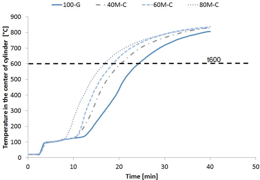
**Fig. 6.** Fire-insulating capacity of 40M-C, 60M-C, 80M-C and 100-G materials
